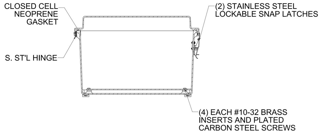
FRONT VIEW WITH COVER REMOVED AND BACK PANEL SHOWN
