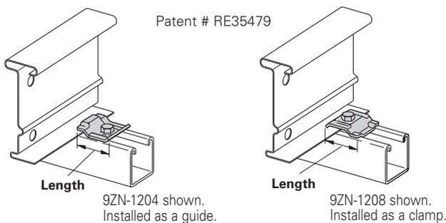
When installing this device as an expansion guide on the outside flange of *Steel Side Rail*, use the Catalog No. **B202** Square Washer in order to properly elevate the guide.
