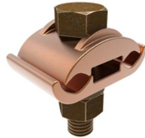
Mechanical Grounding Connector, 2 Copper Cables to 1/4" Thick Bar, 300 kcmil - 500 kcmil, 1/2" Stud.
