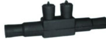
In-Line Splice/Reducer For Direct Burial, 12 AWG - 350 kcmil, 5/16", Dual rated AL9CU for CU or AL.
