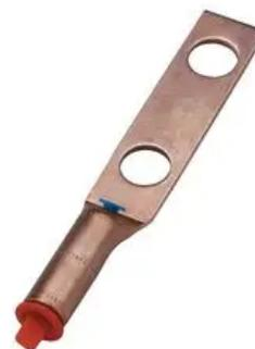
HYLUG™ Copper Compression Terminal for Grounding; 2-Hole; 1/2" Stud; 1-3/4" Spacing; Long Barrel; Accommodates: #8 AWG.
