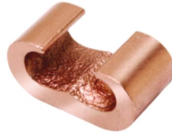
Copper Compression C Connector, 300-500 kcmil, 3/4" Rod (Run) & 6 AWG(Sol) - 2/0 AWG(Str) (Tap).
