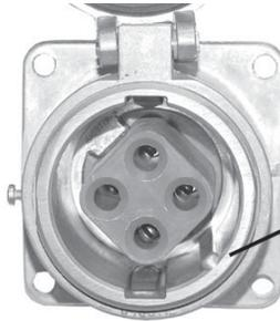
Arktite receptacles have a cast raised rib located inside the receptacle sleeve. The location of the rib is in a specific relationship to the receptacle insulator that houses the contacts.
