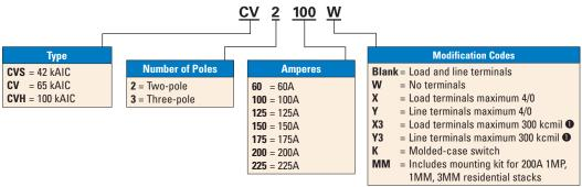
1 300 kcmil options use a terminal shield and add 1.50 inches (38.1 mm) to the length of the breaker.
