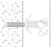
Position the fixture. Insert the proper size screw through the fixture into the top of the anchor and tighten. Be sure screw thread fully engages the anchor body.
