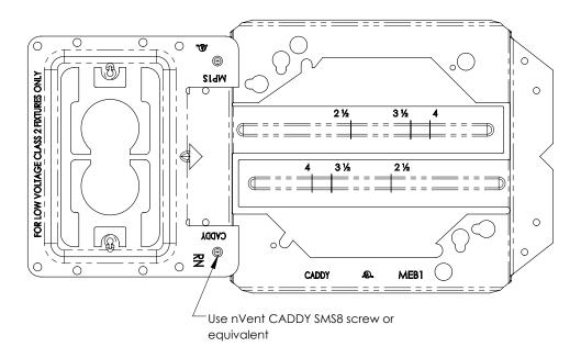
Detail for mounting electrical boxes and Low Voltage Mounting Bracket to the MEB1
