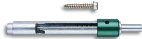
Masonry Screw Anchors must be used with Greenlee masonry screw drill bits, numbers 84484 and 84487, which are a special size to insure secure thread engagement. Standard masonry bit size holes will not provide proper contact with screw threads and may cause masonry anchor screws to pull out.
