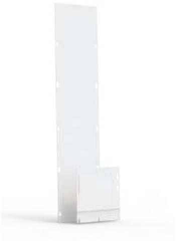
Barrier Panel is used to provide a Type 1 rated barrier between individual Universal Free-Stand Enclosures. Two-piece design mounts on the inside of the enclosure reducing a leak point, installation time and complexity. No additional hardware is required to install barrier once enclosures are bayed together.
