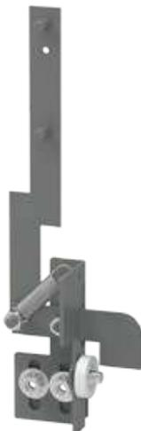
The Operator Release Mechanism provides a connection between the primary door handle orientation and the disconnect device. If the primary door handle is turned to the open position, the disconnect cannot be turned on. Must be used with an Operator Adapter for Preferred Cutouts (sold separately).
