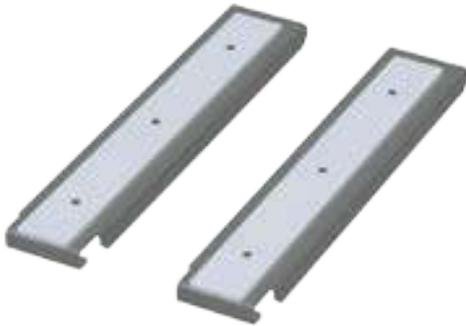
Panel Gliders are used to provide a smooth surface from the front lip of the enclosure to the back panel support. Gliders assist and improve panel installation process. They are intended to be used reusable tools to aid in the installation of panels and removed from enclosure after panel installation.
