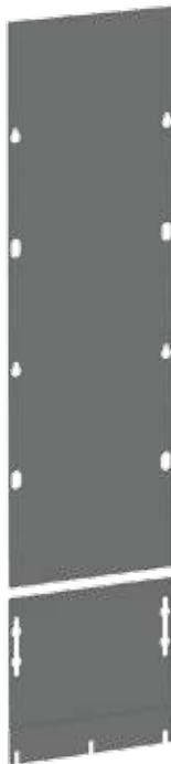
Barrier Panel is used to provide a Type 1 rated barrier between individual Universal Free-Stand Enclosures. Two-piece design mounts on the inside of the enclosure reducing a leak point, installation time and complexity. No additional hardware is required to install barrier once enclosures are bayed together.
