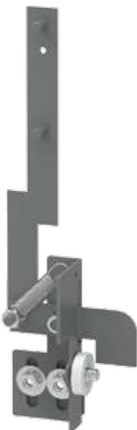
The Operator Release Mechanism provides a connection between the primary door handle orientation and the disconnect device. If the primary door handle is turned to the open position, the disconnect cannot be turned on. Must be used with an Operator Adapter for Preferred Cutouts (sold separately).
