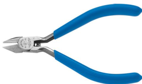
These Klein Tools Electronics pliers feature a sharp, pointed nose with extra narrow jaw for delicate work in tight spaces. The short jaws have induction-hardened, beveled, full-flush cutting knives for close precise cuts and durability. The handles are spring-loaded for self-opening action and plastic dipped for comfort and ease of identification.
