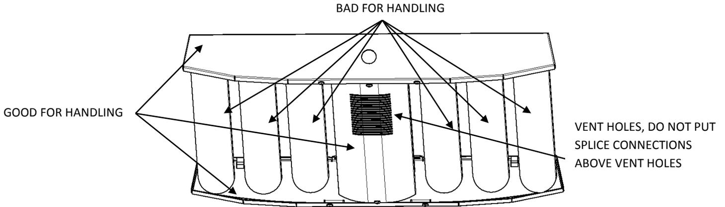
When handling the fixture during unpacking and installation do NOT use LED Modules for carrying/support. DO use the center channel and end caps for carrying/support
