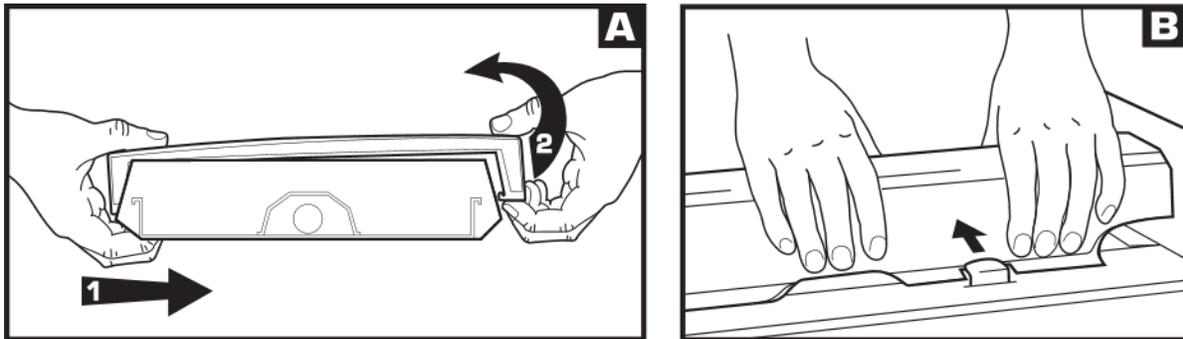
A: Remove diffuser from housing by sliding diffuser to one side, then lift up opposite side over flange as shown.
