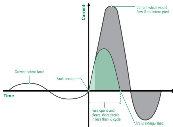
Figure 13 – Current-limiting Fuse
