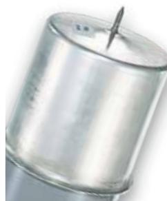
Current-limiting E- and R-rated fuses are equipped with a mechanical indicator or striker pin that protrudes through the fuse cap upon operation of the fuse. This provides visual identification of a blown fuse and can be used as a trigger for external devices.
