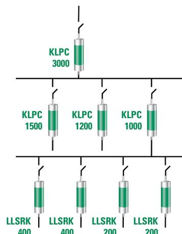
Figure 9 – Example of Selectively Coordinated Fused System
