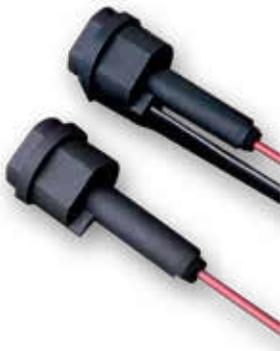
Fuse holders are rated up to 10 amperes at 300 volts and are equipped with 7" 18 AWG leads. Order part number LHR000 for two leads, and part number LHR001 for one lead; with the other terminal used for insertion of 18 AWG ballast lead.
