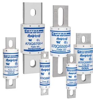
A70QS Amp-Trap® high speed fuses were developed in response to the need for improved overall performance of 700V semiconductor fuses for new equipment requirements. A70QS fuses have lower I<sup>2</sup>t for better protection, longer life when subjected to cyclic loading, plus lower watts loss. A70QS is the best choice to protect dynamic solid state equipment such as motor drives, UPS, etc.
