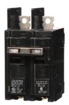
Siemens Low Voltage Molded Case Circuit Breakers General Purpose MCCBs - Type BQ, 2-Pole, 120/240VAC are Circuit Protection Molded Case Circuit Breakers. 2-Pole Common-Trip circuit breaker type BQ. Rated 120/240V (030A) (AIR 10 kA). Special features: Load side lugs are included.
