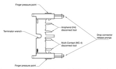
If the disconnect tool is not available, insert a #3 Phillips screwdriver into one hole, and rock that side of the drop connector out. Then, insert the screwdriver into the other hole and pull the connector out entirely.
