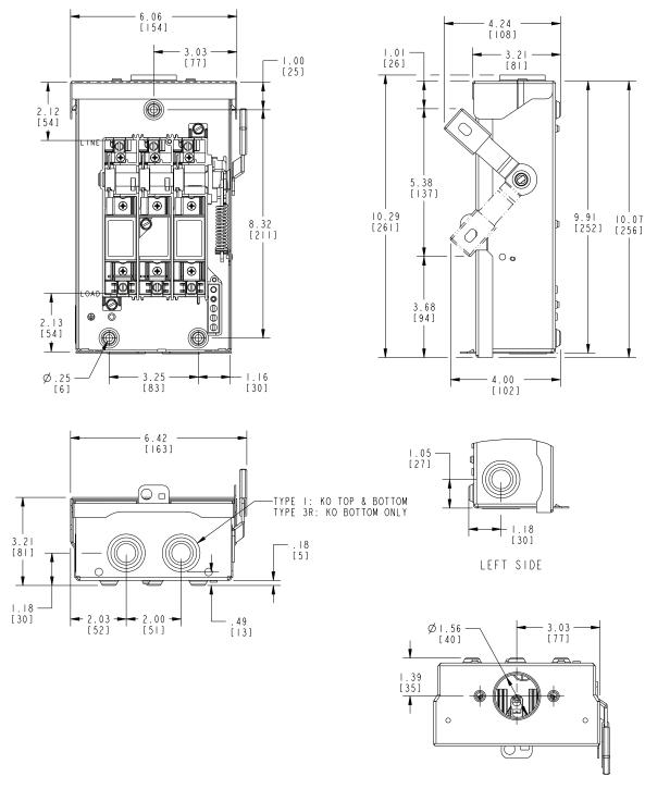
TYPE | ENCLOSURES: COLD ROLLED STEEL .045" THICK FINISH: ANSI GREY #61 PAINT
