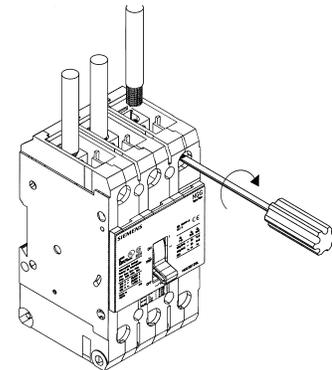
It is possible to remove factory installed lugs to allow customer-supplied connections.
