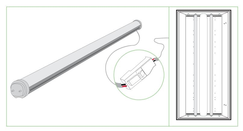
STEP 4: Utilize the existing tombstones to hold the Ti Tubes. Once the tubes are held in place simply connect the quick connects and push the lines back into the wire compartment.
