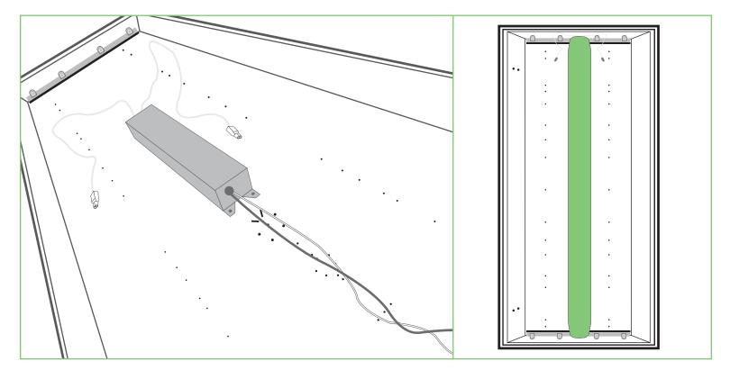
STEP 3: Once the ballast is removed replace it with the ESL Vision Quick Connect Driver. The driver is designed to fit in the same location as the previous ballast. Pull the DC lines to the end of the wire compartment. Replace the ballast cover.
