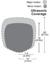
For best performance, Wattstopper recommends using this sensor in spaces no larger than 15' x 15'.
