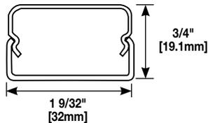
Receptacles prevent the accidental insertion of foreign objects into receptacles reducing the risk of shocks or electrocution. Meets 2014 NEC section 406 requirements. Available in 3' [914mm], 5' [1.5m] and 6' [1.8m] lengths with 6" [152mm] receptacle spacing. 15A tamper-resistant receptacles. 3-wire, #12 THHN (1 hot, 1 neutral, and insulated ground conductor). .040" [1.0mm] steel housing. Packed 2 per carton. Each unit supplied with one (1) Coupling and two (2) Blank End Fittings.
