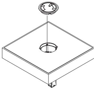
**Step 3b For ABPLUG6 & ABPLUG8:** Remove poke-thru unit from floor by bending tabs inward and pulling unit up.
