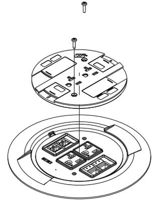
**Step 3** Attach abandonment plate with two screws provided.
