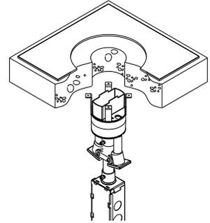
**Step 2b For ABPLUG6 & ABPLUG8:** Remove cover assembly from Poke-Thru by removing two (2) 8-32 screws and lifting cover off.
