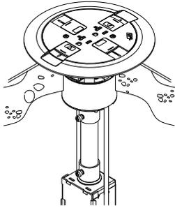
**Step 2a For ABPLUG3 & ABPLUG4:** Remove slide holder assembly and the internal gasket. Disconnect power and communications devices and remove flange.
