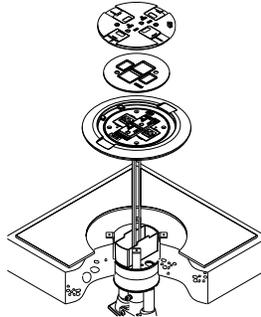
**Step 3a For ABPLUG3 & ABPLUG4:** Remove poke-thru unit from hole.
